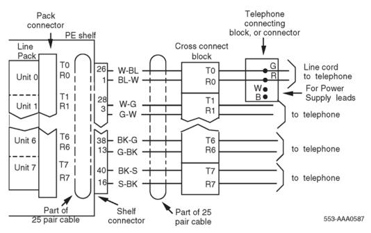
Figure 63: Meridian Modular Telephone cross-connections
