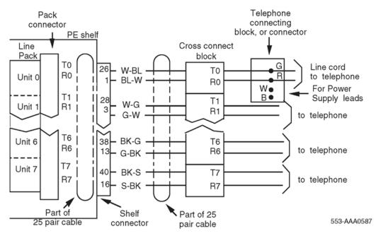
Figure 24: M2016S telephone cross-connections
