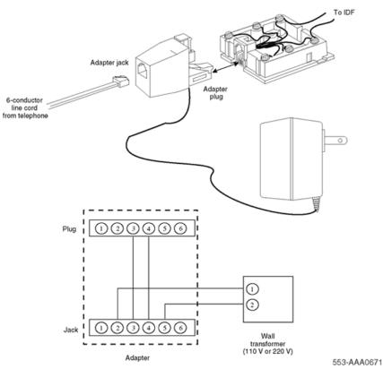
Figure 37: Wall transformer connections
