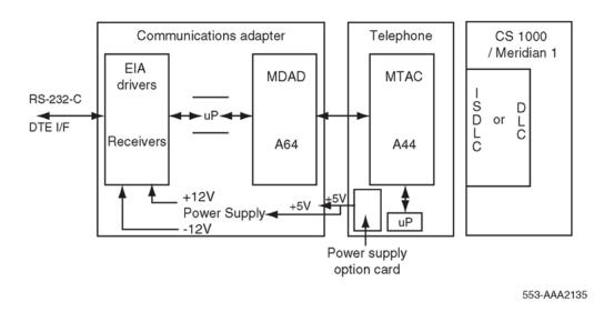
Figure 57: Block diagram of MPDA and Meridian Modular Telephone
