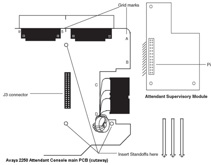
Figure 9: Identifying the correct grid positions on the main PCB and attaching the ASM
