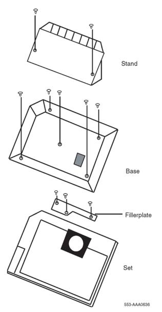
Figure 64: Exploded view of the M2616/M2016S/M2216ACD telephone
