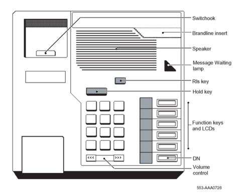
Length: 8.42 in. (216 mm) Width: 8.42 in. (216 mm) Height: 3.61 in. (92.6 mm) Weight: approximately 2.65 lbs (1.1 kg)
