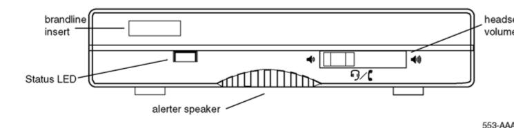
Figure 18: PC Console Interface Unit
