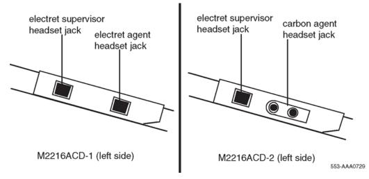
Figure 55: M2216ACD-1 and -2 left side showing headset jacks
