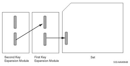
Figure 81: Key Expansion Module connections (bottom view)
