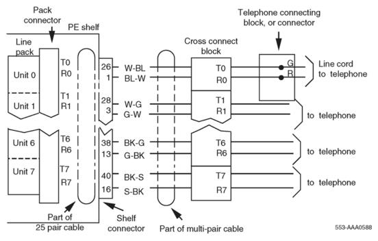
Figure 62: M2317 digital telephone cross-connections
