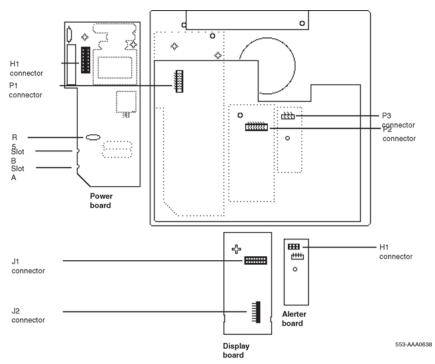
Figure 70: M2006/M2008 telephone and option boards
