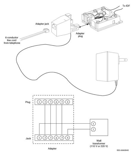
Figure 72: Configuration of a local plug-in transformer
