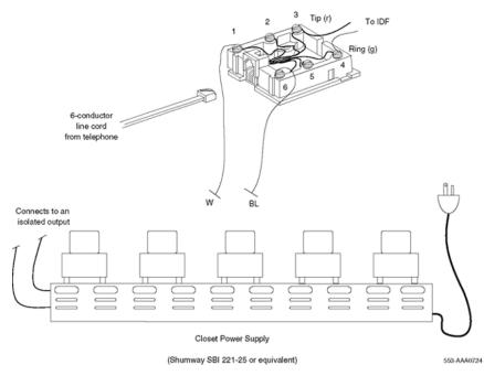
Figure 102: Closet Power Supply configuration
