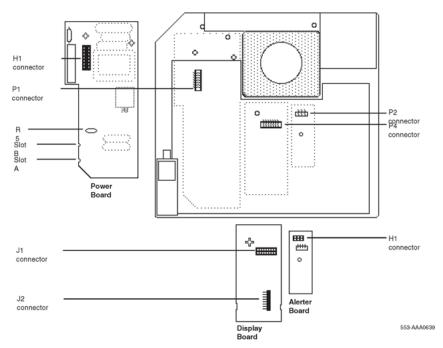
Figure 71: M2616/M2216ACD telephone and option boards
