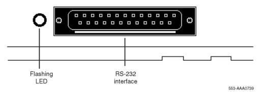
Figure 67: Back of telephone showing MCA
