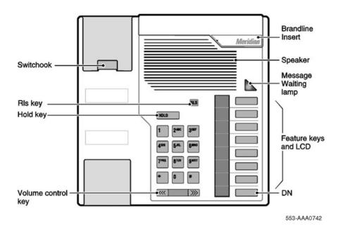
Length: 9.75 in. (251 mm) Width: 9.45 in. (237 mm) Height: 3.64 in. (92.6 mm) Weight: approximately 2.65 lbs (1.1 kg)
