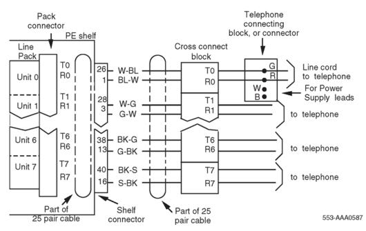
Figure 23: M2016S cross-connections.
