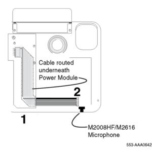
Figure 74: Ribbon cable placement
