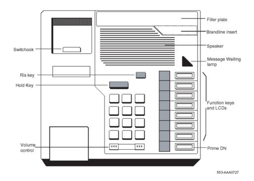
Length: 8.42 in. (216 mm) Width: 8.42 in. (216 mm) Height: 3.61 in. (92.6 mm) Weight: approximately 2.65 lbs (1.1 kg)
