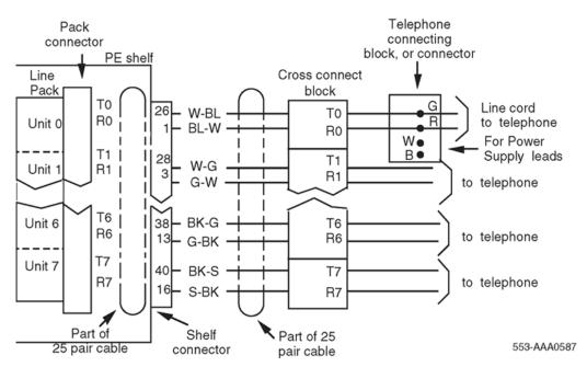
Figure 61: Meridian Modular Telephone cross-connections.
