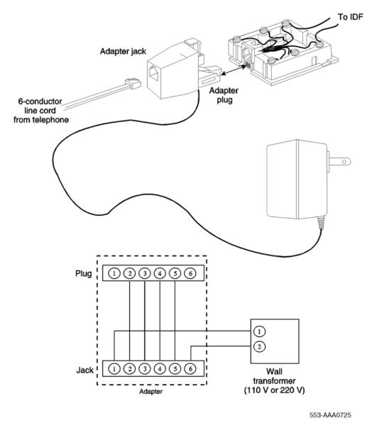
Figure 21: Configuration of local plug-in transformer
