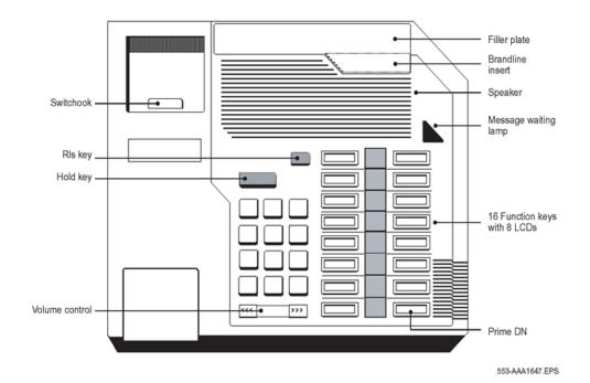
Length: 9.75 in. (251 mm) Width: 9.45 in. (237 mm) Height: 3.64 in. (92.6 mm) Weight: approximately 2.65 lbs (1.1 kg)
